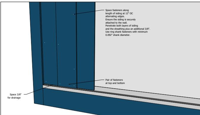
When bridging floor assemblies, fasten trim and vertical lap siding with a minimum of two fasteners in the upper portion of the rim board and another pair of fasteners into the lower portion of the rim board. Avoid fastening into the bottom or top plates.
